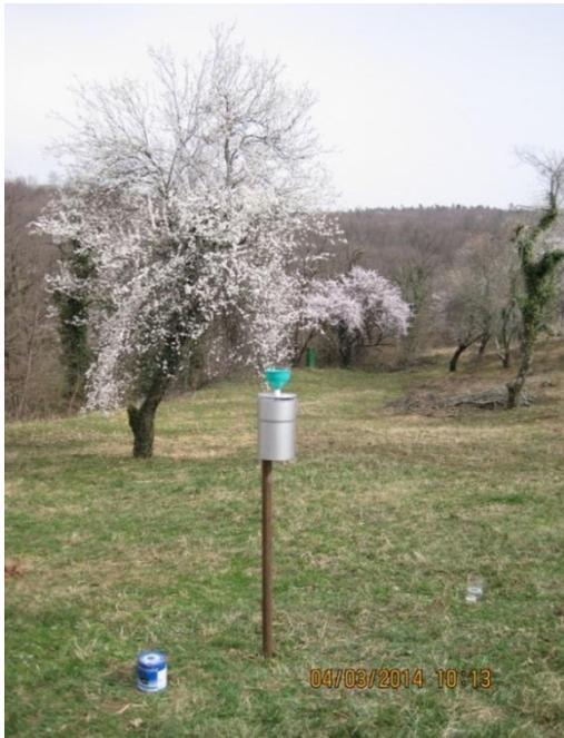
Figure 4 Palmex rain collector (2014/2240
