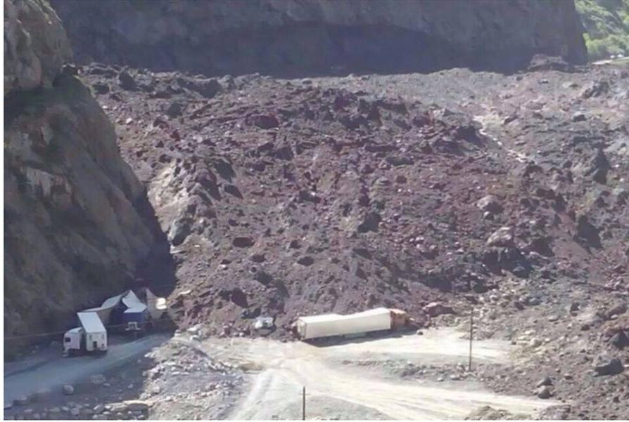
Fig.1. The landslide in Dariali Gorge in northern Georgia, on the Greater Caucasus range 17 May 2014. It severed the road connecting Georgia and Russia causing large economic losses and several deaths
