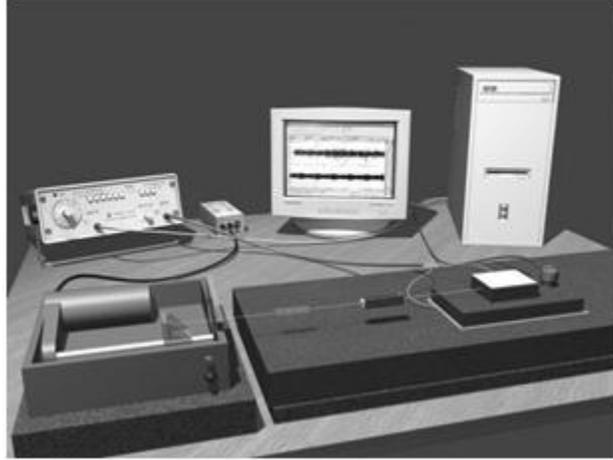
Fig.1. The scheme of laboratory installation for studying stick-slip synchronization.
