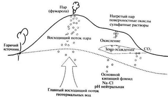
Fig.5b. A schematic illustration of the vertical directed main geothermal flows; hot gazer (left); main boiling fluid Na-Cl, pH neutral; hot steam, surface oxide, solutions; oxidation; zone of precipitation [10].
