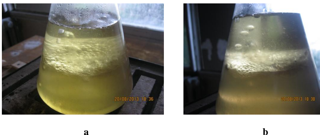
Fig. 8. Three-layer thermodynamic system – glucose syrup layer (bottom), thick intermediate bubbles and population (IP) layer, oil layer (it’s well seen group of large air- bubbles), thin intermediate bubble and IP layer, and air-steam layer (top): (a) photograph shows oblique view of the solution topography; (b) photograph shows view from side (after 2 min).
