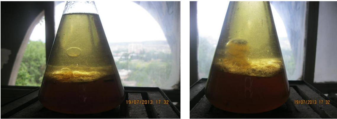
Fig. 9. Photographs show the same thermodynamic system as in Fig. 8, but here glucose solution colored by coffee: (a) it is well seen two large air bubbles fast vertically ascend upward ( \sim 40 cm/s); (b) large bubbles made their way through the thick intermediate bubbles and population (IP) layer (after 14 sec).
