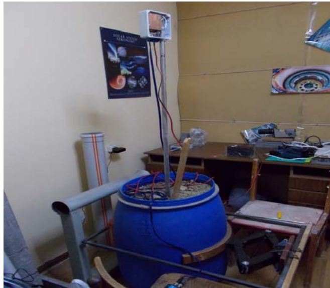
Fig.5. Landslide creep modeling and accompanying AE registration
