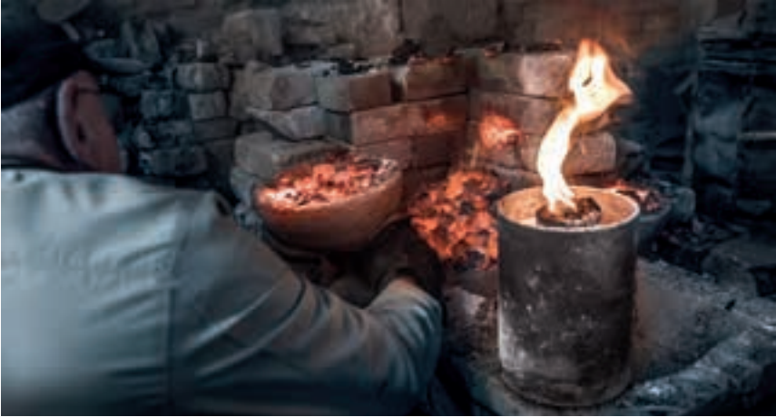
Fig. 5. Master can take Sakhoveli-type crucible with molten bronz mass in his hands during a work process.
