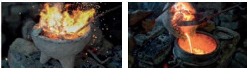
Fig. 4. Process of casting bronze with an experiment conducted in my laboratory in Gori.
