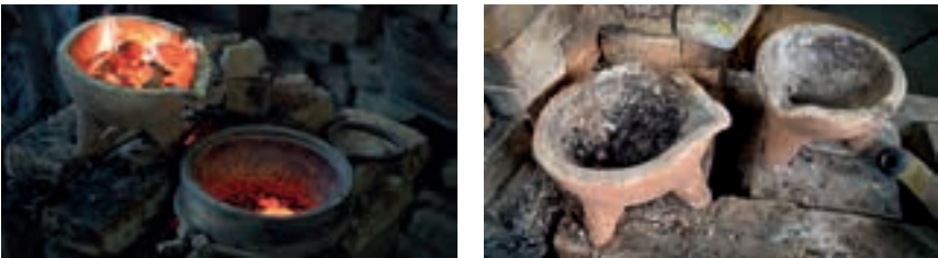
Fig. 6. Experimental crucibles after completion of the metallurgical process.
