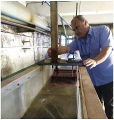
Fig. 7. Debris flow regulation elastic barrage during the laboratory tests
