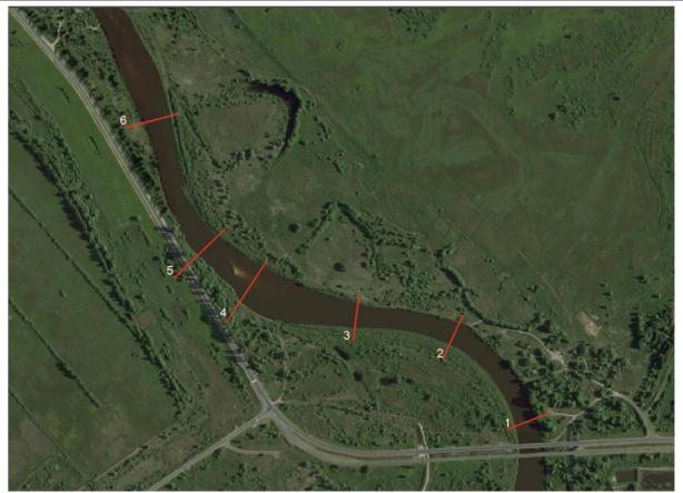
Fig. 1. The design section of the Pripyat River (Cross-sectional numbers in numerals)
