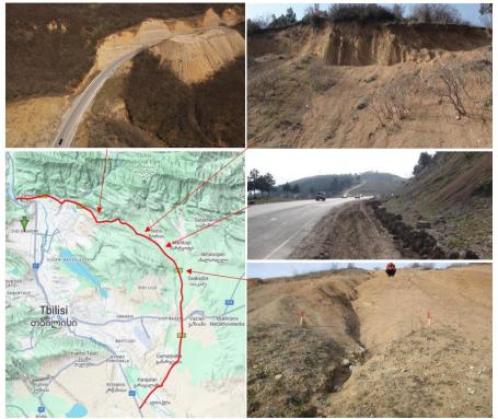
Fig. 1. Schematic illustration of eroded sections of the Tbilisi bypass
