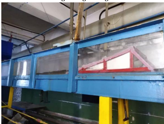
Fig. 9. Debris flow regulation elastic barrage during the laboratory tests
