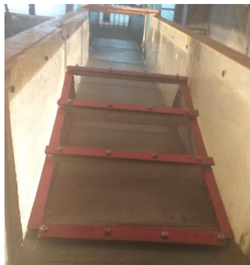
Fig. 8. Model of the elastic debris flow-regulating barrage in the hydraulic duct
