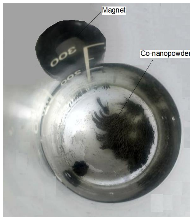
Fig. 2. Received Co magnetic powder
