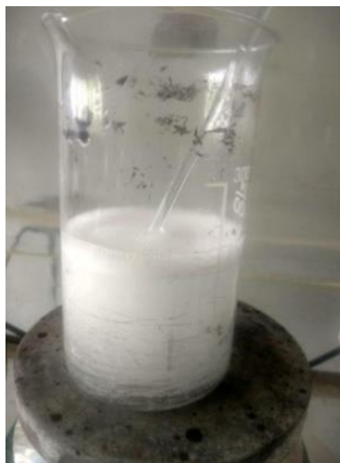
Fig. 1. The picture of Co particles deposition from Co chemical solution. Solution became colorless, i.e. depleted from Co ions.
