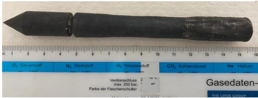
Fig.13. Photo of the sample obtained by HSWC compaction.
