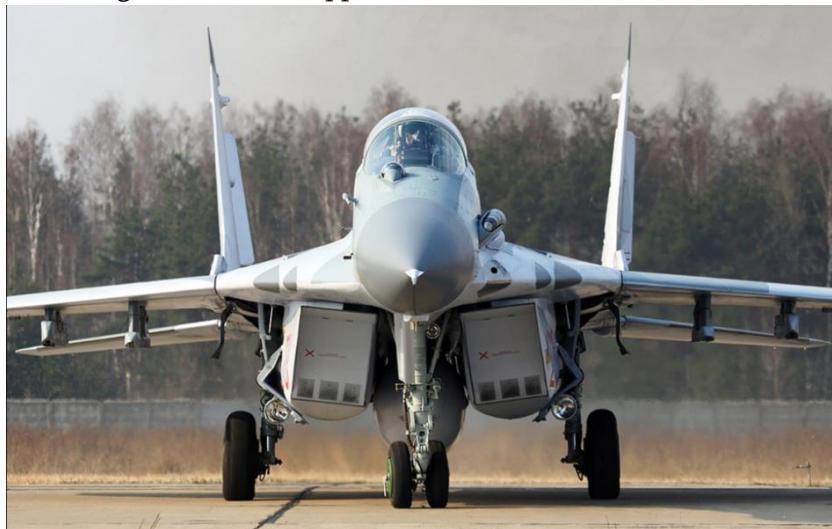
Fig. 7. Engines of fighter MIG-29CMT with closed protective panels
