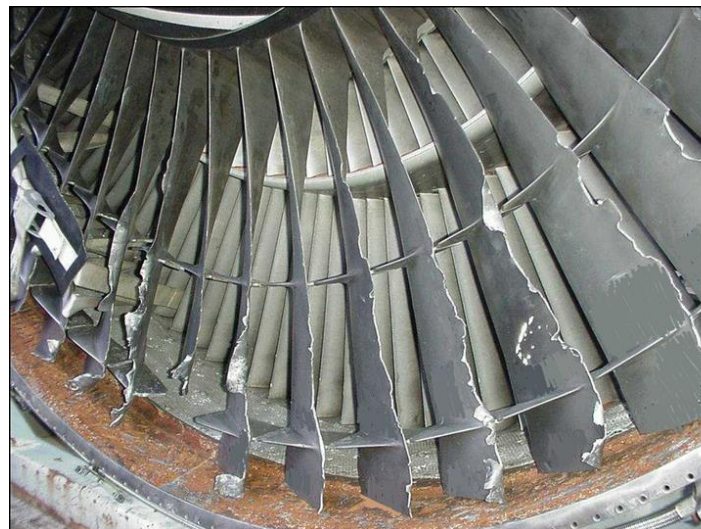
Fig. 4. The gas turbine engine compressor after collision with foreign objects
