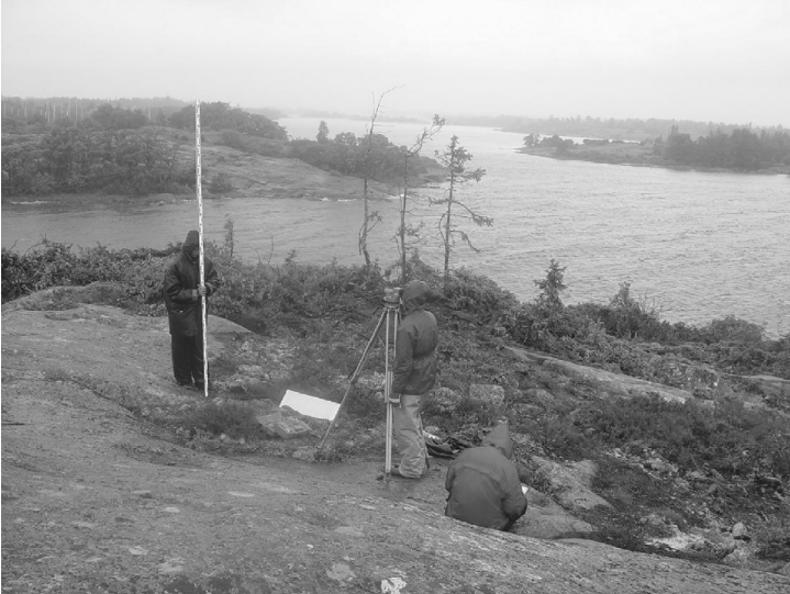
Fig 8. Expedition members working with the level machine in order to get the coordinates for the rock carvings. Photographer: Alopaeus, Harry.
