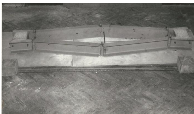
Photo 8. Experimental installation for the creation of prestressed concrete beams reinforced with BPA
