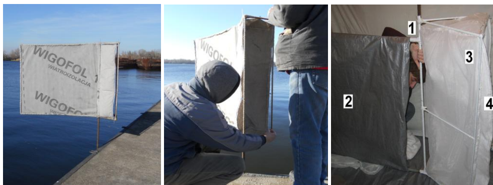
Fig. 1. a) aerosol trap; b) replacement of filter for following sampling of substance from trap; c) trap installation (1 – triangle frame, 2 – textile of stabilizer tail, 3 – outer layer of filter textile, 4 – inner layer of filter textile)
