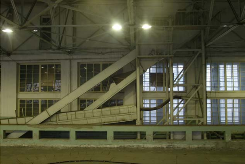
Fig. 3. Hydraulic chute for modeling mudflows
