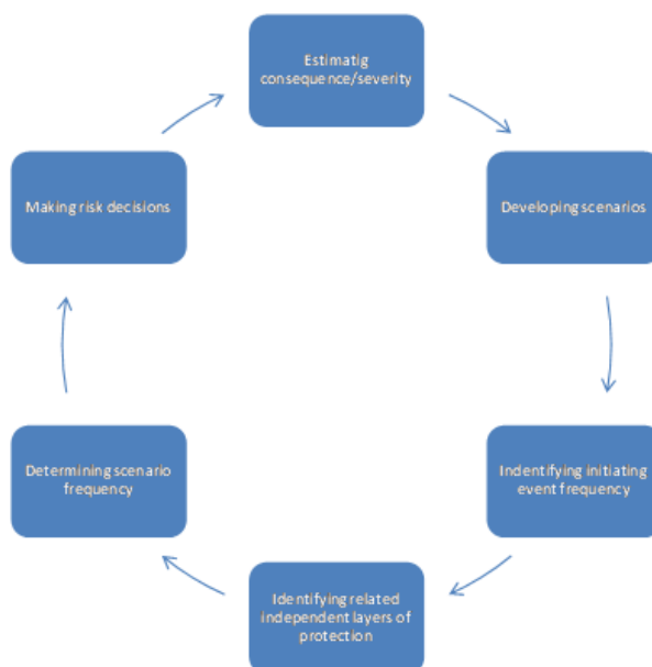
Figure 6. Steps of Layers of protection analysis
