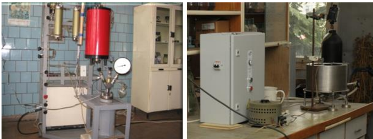
Laboratory Supercritical Fluid Extractor (left) and ultrasound extraction (right)
