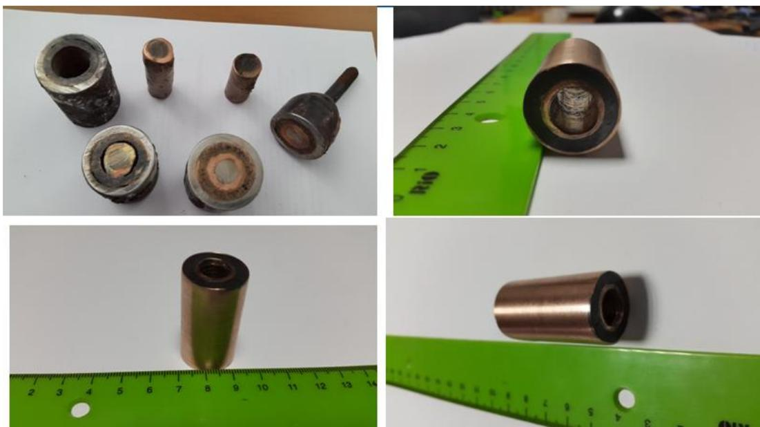
**Fig. 7. Cu-MgB<sub>2</sub>-Cu superconducting tubes**
