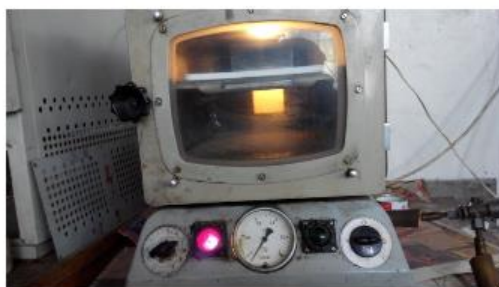
Fig.3. The vacuum cabinet with sample under testing
