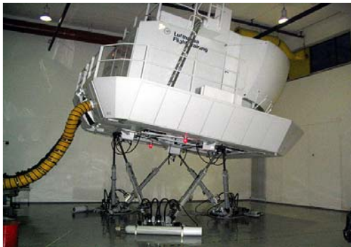
Fig.1 Stewart platform used for flight simulator
