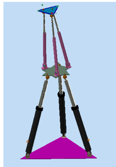
Fig.3 Structure of paired tripod mechanism
