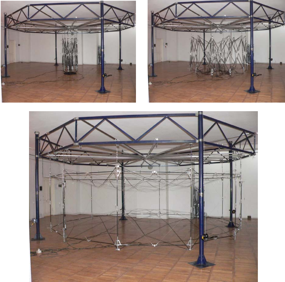
Figure 7 Photo of the 6 meter deployable reflector antenna having the ring with “V-fold bars”
