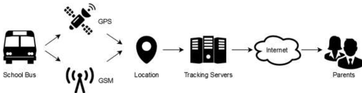
Fig. 5. School bus GPS tracking system
