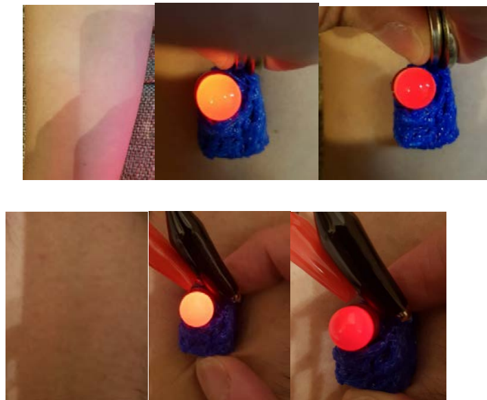
Figure 14. On the top is a forearm of a female and at the bottom there is a leg of a male case. From left to right; Left: Without using device, mid: using device in a place that there is no vein (we use it as a reference indication), right: when we put device on the top of the vein (as you see the current and following that the intensity of indicator decreases).
