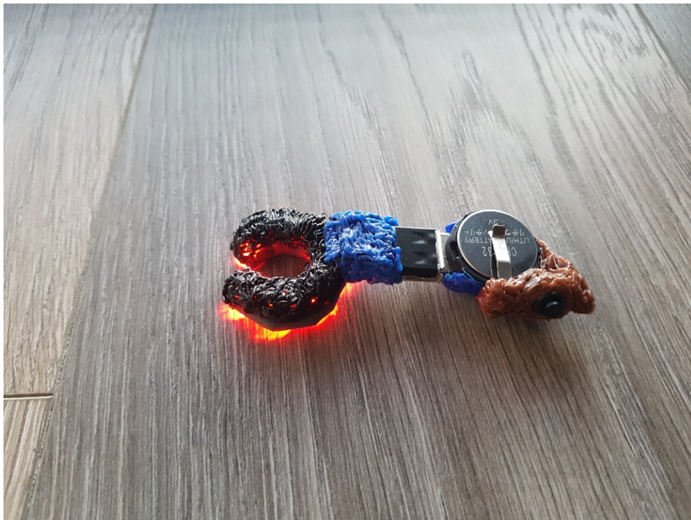
Figure 72. Model B; 7 Leds in parallel array with one 3 volts' battery.
