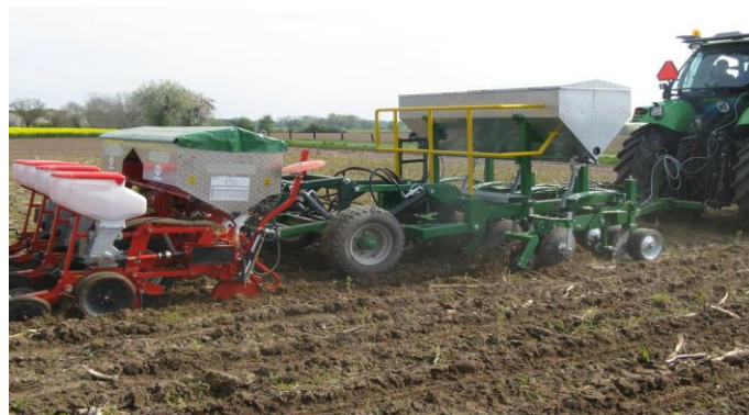
Fig. 4. The machine for simultaneous maize sowing and fertilization
