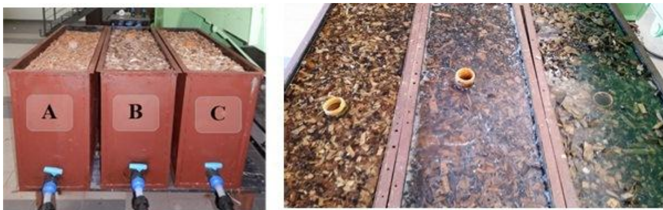
Fig. 1 Physical denitrification bioreactors models with different fillers (A – deciduous woodchips; B – coniferous woodchips; C – mixed woodchips)
