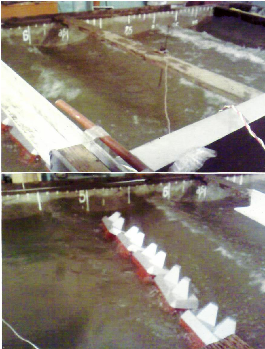
Fig. 3. Preliminary experimental study of the wave damping structures system proposed in the project in hydraulic laboratory
