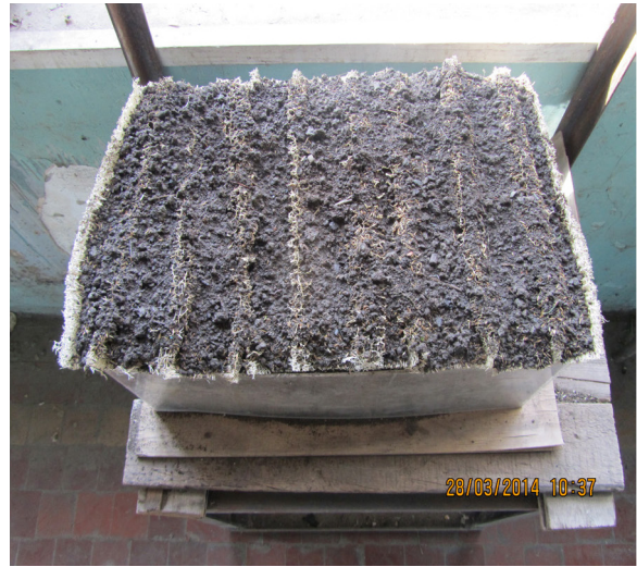
Fig. 3. Beginning of the laboratory experiment carried out on geomat „Luffaeromat”
