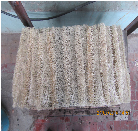
Fig. 3. Beginning of the laboratory experiment carried out on geomat „Luffaeromat”
