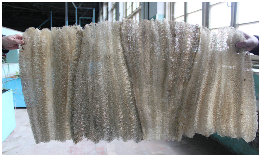
Fig. 2. Overall view of geomat „Luffaeromat” created as a result of longitudinal section and connection of Luffa fruit
