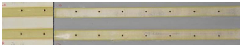
Figure 14. Aluminium panels after plasma paint stripping, left-test panel 7075-T6, and right-test panel 2024-T3.
