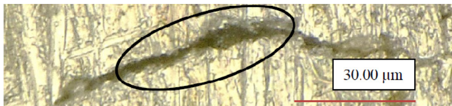
Figure 12. Close-up view of unknown residues in the cracks(circled) of the test panel 7075-T6 aluminium.
