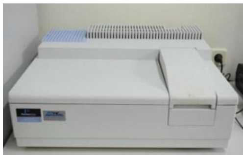
Figure 8. Double-ray scanner-spectrometer Lambda 35 operates in Vis. And UV regions of the spectrum (190 – 1100 nm). Its function is objects' quantitative and qualitative analysis
