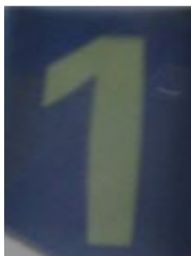
Figure 4. The image generated by a photomasked UV irradiation ( \lambda = 365 nm) of the PMMA film doped with hybrid compound I.
