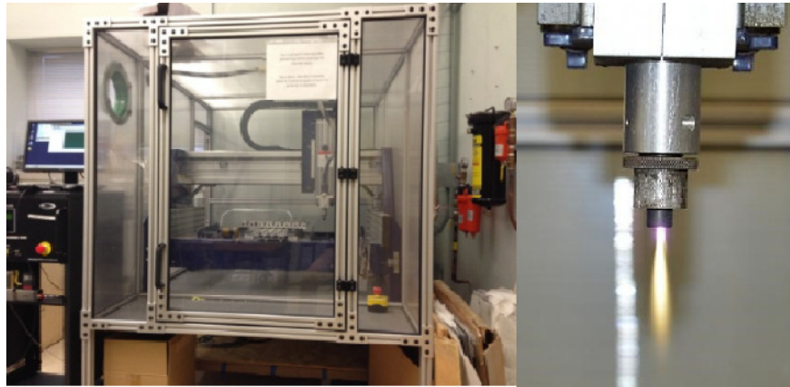
Figure 13. Front view of APS plasma flux paint removal system with 3D robot and exhaust cabinet (left). Close up of the plasma plume (right).
