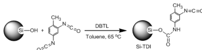
Figure 2. Toluene diisocyanate functionalization of SNPs.
