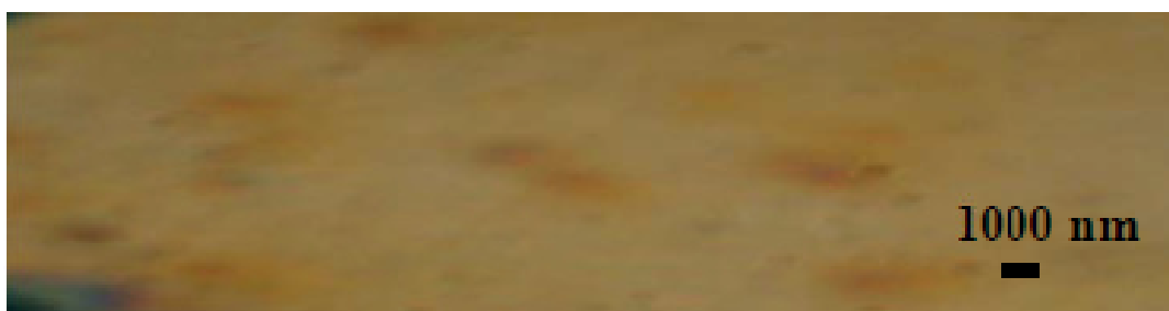
Figure 5. Microstructure of SiO 2 + TiO 2 + ZrO 2 + Au 0.03 film with thickness h \approx 200 nm on Si (100).
