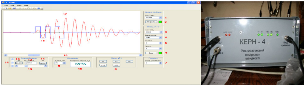
Figure 3. The window illustration of data treatment of elastic waves velocities measuring by the echo-impulse method on frequency f_{\parallel} \approx 1.11 MGz, f_{\perp} \approx 0.43 MGz and appearance of ultrasound computer device KERN-4.
