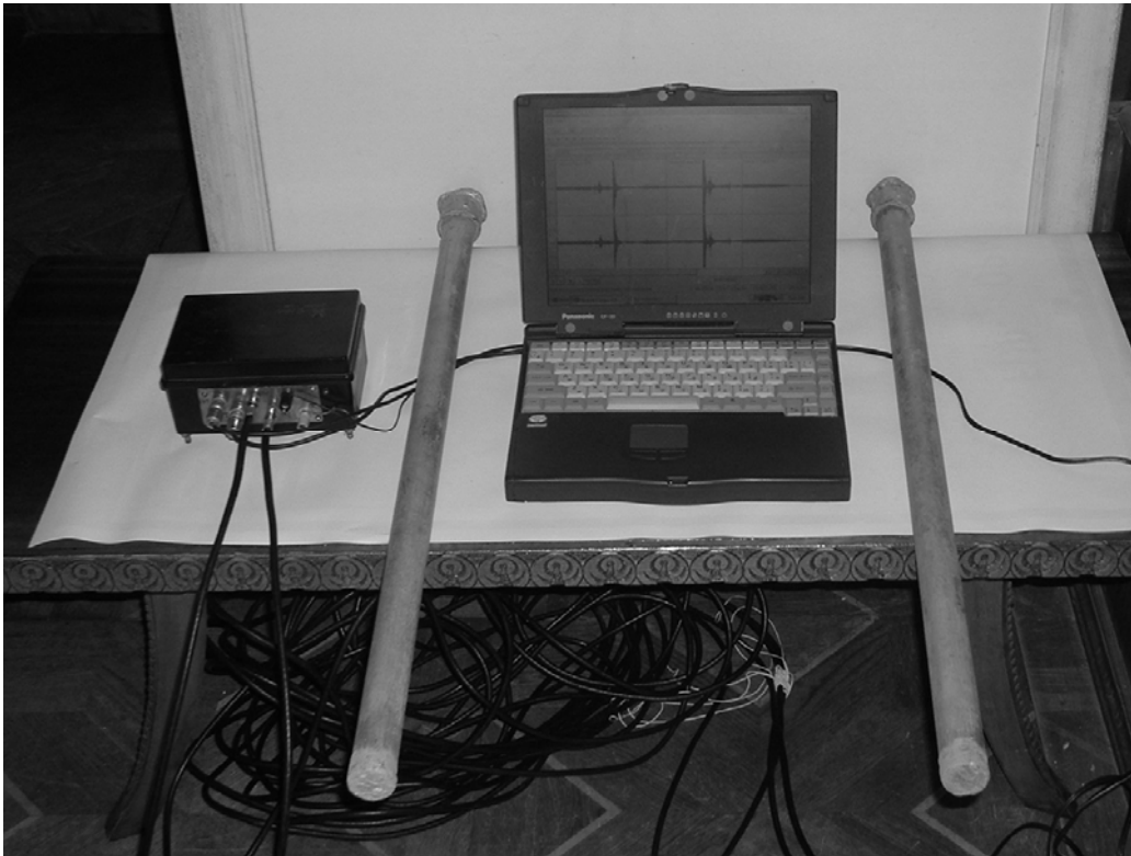
Fig. 3. The field acoustic system for debris-flow EWS, including the electronic unit with amplifiers and filters, two sensors and notebook
