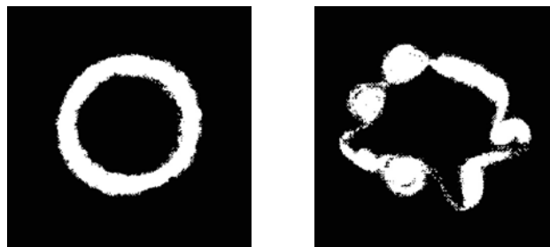
Fig.2. Hollow electron beam [19] Distance from cathode is 1cm (left) and 8.7cm (right)
