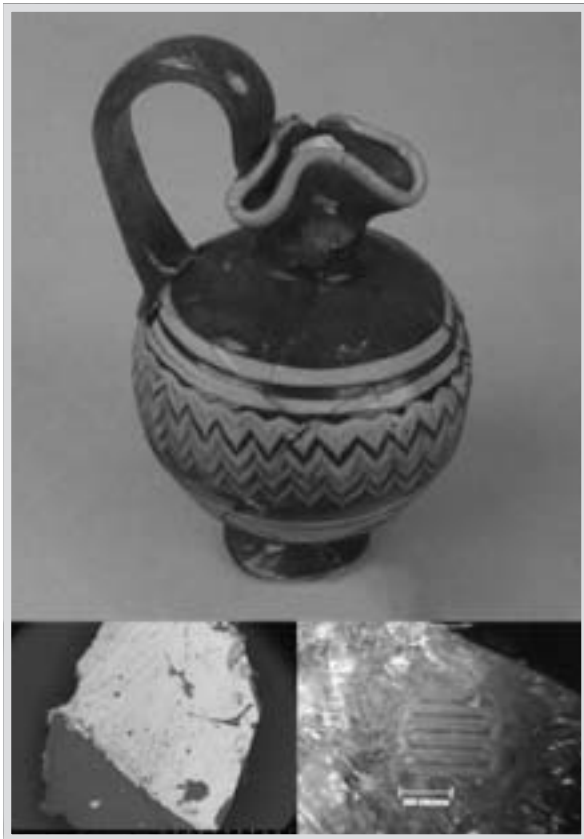
Figure 6. . The topmost image is of LRN6675, a blue vessel, before treatment. On the lower left is an electron micrograph of sample LRN6675, a pale blue shard. The darker areas are most likely conservation materials. The lower right hand image shows the sample after laser ablation.
