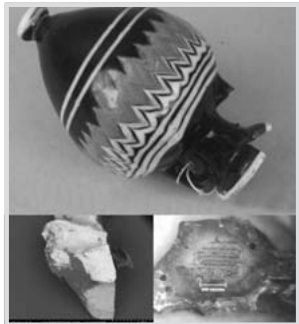
Figure 5. The topmost image is of LRN6674, a blue vessel, before treatment. On the left is an electron micrograph of sample LRN6674b, half of a large, clear-blue shard. The darker areas are most likely conservation materials. The lower right hand image shows the sample after laser ablation.
