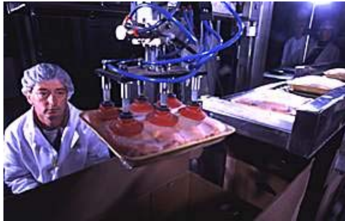
Fig.1.12 Belt Manipulator picks up packaged chicken from a conveyor belt.
