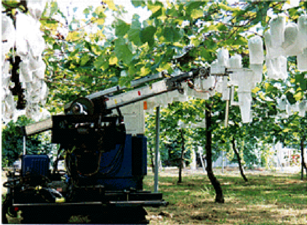
Fig.1.6 Multi-Operation Robot for Grapevine (Bagging operation).
