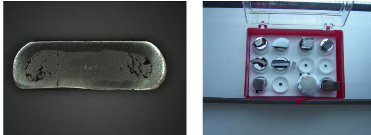
Figure 4. Photograph of SC / SHS compacted Ti / Al / B samples of different shape.
