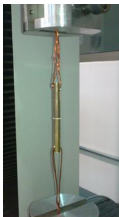
Figure 2. Coating adhesion testing by MTS machine: coated samples were loaded as shown in the highlighted section of the apparatus.
