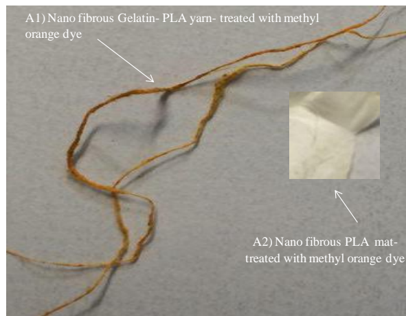
Figure 6. Gelatin + PLA yarn and PLA sheet after dyeing with methyl orange.
