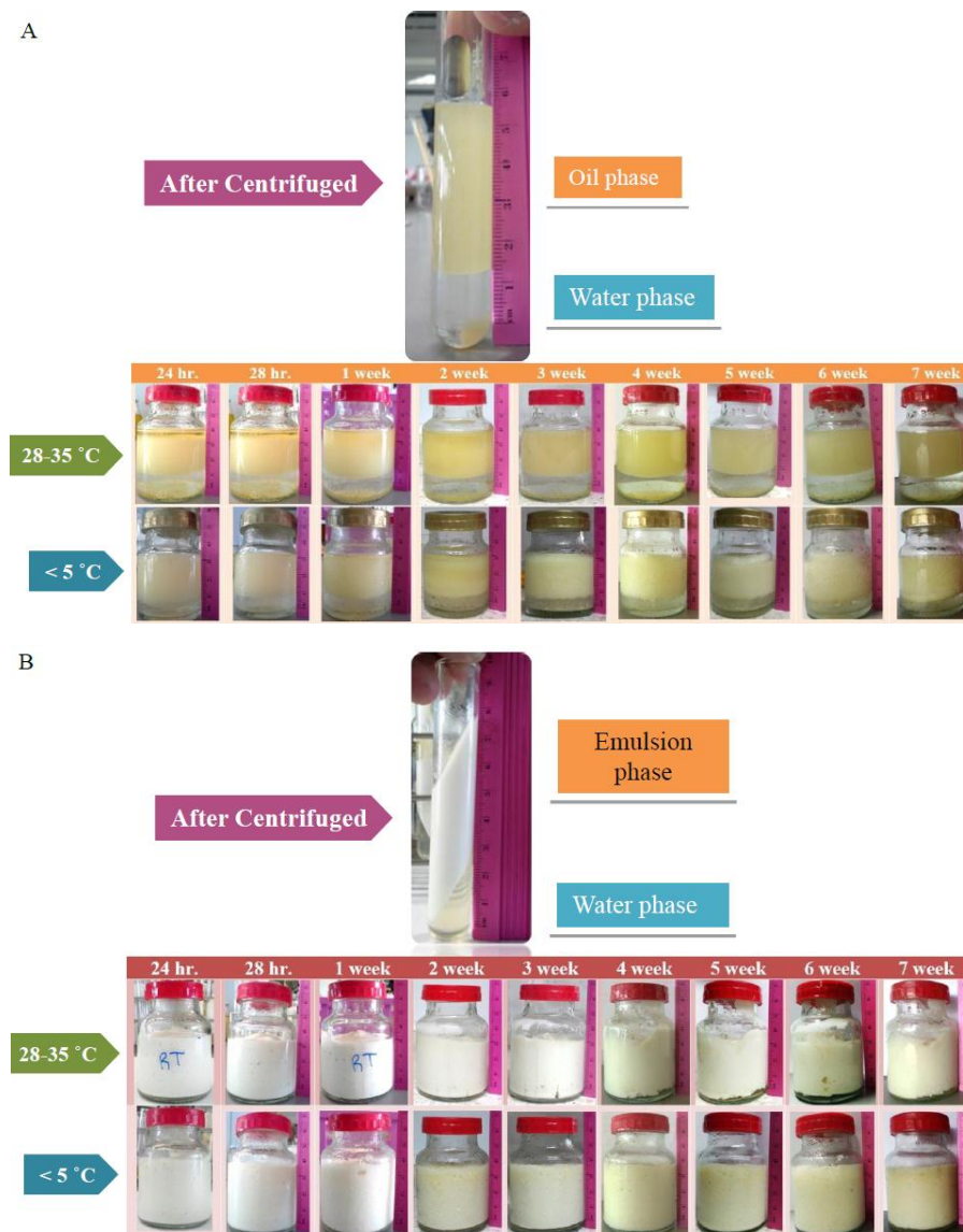
Figure 2. A) Water: RBO (with PG 1.5 SF R0.05 2.5 wt. %) in a ratio of 50 : 50; B) Water (with gum Arabic 5 wt. %): RBO (with PG 1.5 SF R0.05 5 wt. %) in a ratio of 50 : 50.
