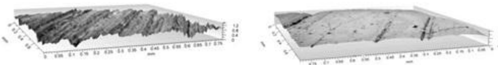
Figure 9. Images before and after coating operation obtained by a confocal microscope.
