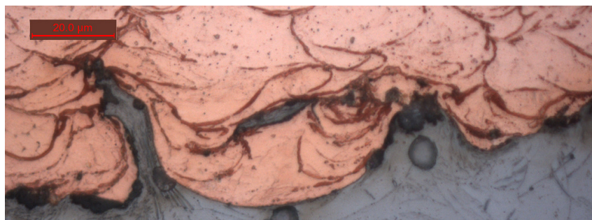
Figure 7. Structure of coating / substrate interface.
