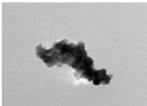
Figure 4. TEM image of the sample ZnCr 0.4 Fe 1.6 O 4 .
