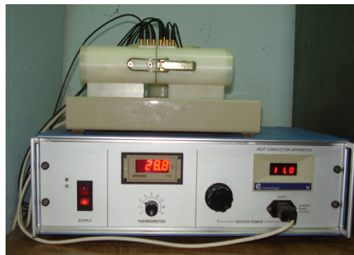
Figure 3. Thermal conductivity test equipment.
