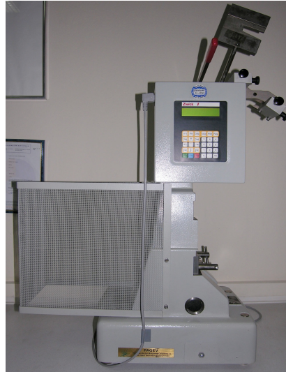
Figure 4. Charpy impact test equipment.
