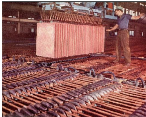
Figure 11. Anodes handling system.
