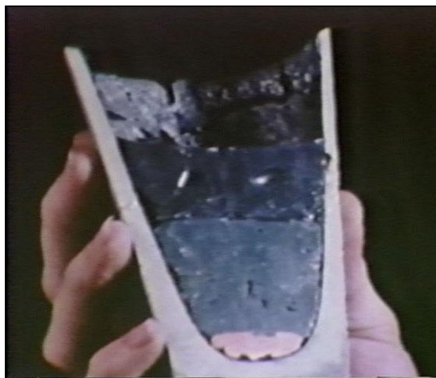
Figure 2. Formation of three immiscible layers: slag, matte, and metallic copper when melting copper sulfide concentrate under certain conditions.
