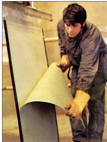
Figure 14. Manual stripping of zinc cathodes from blanks.
