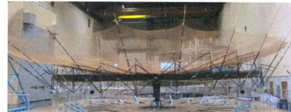
Figure 3.5-7: Large Deployable Antenna EQM in deployed configuration
